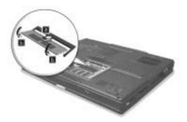
4 Replace the memory compartment door, and fasten the screw. The computer automatically detects the new module and reconfigures the memory.
